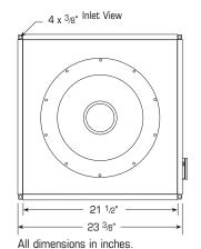
Unit Specifications: Housing Metal Thickness - 16 Gauge Approximate Weight - 95 lbs.
