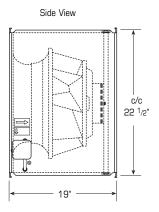
Outlet Velocity (fpm) = CFM x 0.312Tip Speed (fpm) = RPM x 4.869
