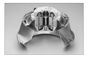
All FSD Series fans are powered by an external rotor motorized impeller. This design provides excellent heat dissipation even at low rpm. All of the FSD Series fans are 100% speed controllable through voltage or frequency reduction allowing for precision balancing of systems. FSD Models 18 - 22 can be supplied with 115/1/60 or 208-230/1/60 motors. FSD22 can also be supplied with a 230-460/3/60 motor. Model FSD26 is supplied with a 230-460/3/60 motor.
