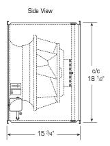
Outlet Velocity (fpm) = CFM x 0.464 Tip Speed (fpm) = RPM x 3.717
